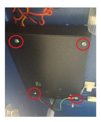
3. Loosen those four screws (see the red arrow) which fix the control panel, and disconnect all the cables connected (see the red circles) refer to below picture.
